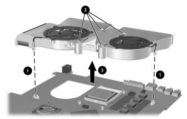
Removing the Heat Sink
